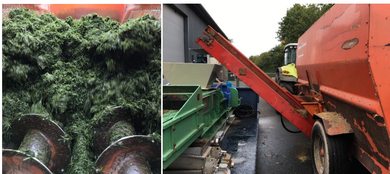
Figure 1. Left photo: Mixing of freshly cut grass in Seko mixer unit. Right photo: Feeding of Twin Screw Press from Seko mixer unit.
