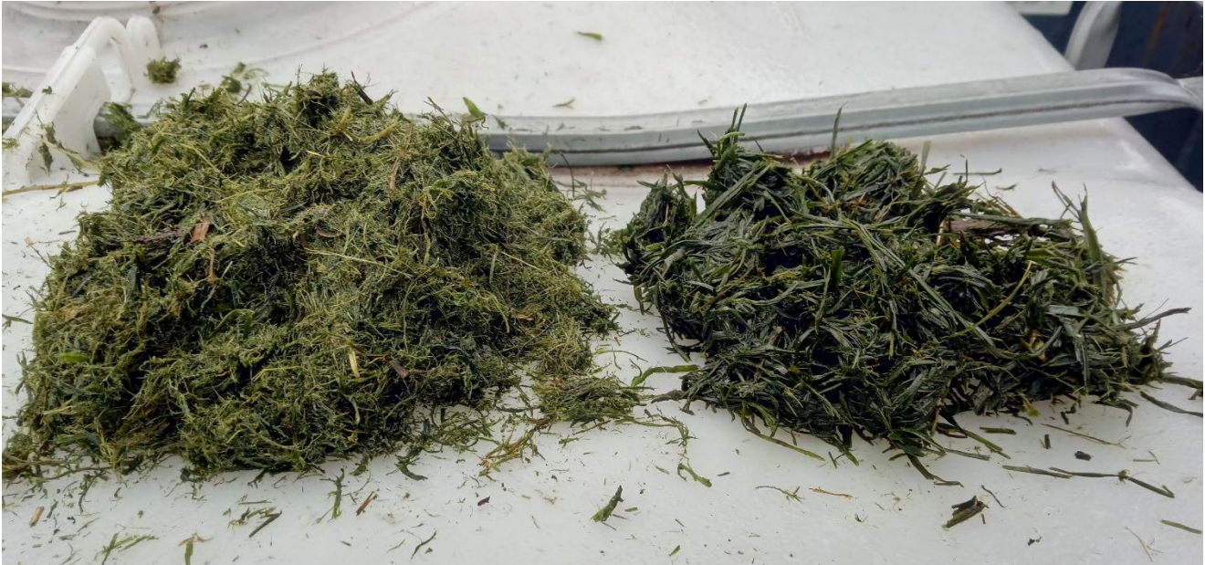
Figure 2. Left: Grass fiber fraction after treatment in Twin Screw Press. Right: Fresh grass after treatment in Seko mixer.
