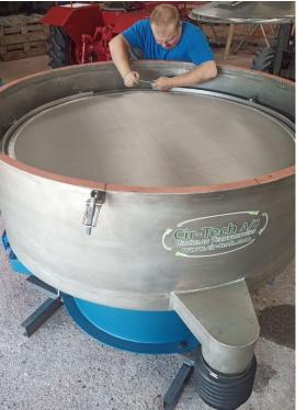
GS Vibro screen the screen is a compact and simple screen, which by means of strong vibration separating particles from liquid or dry fractionation. The screens are available in many sizes and can be combined with two screens on top of each other. this compact and simple mounting makes the machine very robust and secure and gives it longevity. All media-affected parts are made of stainless steel.
