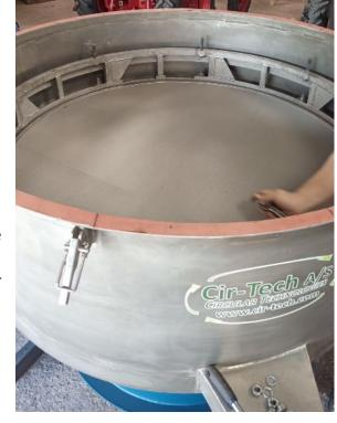
The GS Vibro screen is available in both single and double decks With a screen mesh of 100 microns. it is an advantage to mount a filter with larger holes at the top to take the largest amount of material and the fine filter at the bottom to achieve the highest capacity and gentle sifting
