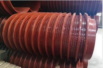
The filter has round holes and is reinforced for long service life. The holes are conical, to prevent material trapped from blocking them. Filters with 3 and 4 mm openings are available as standard.
