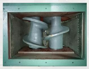
The inlet is fitted with a heavy duty grating for rapid draining of fluids. The considerable increase in screw threads ensures a high level of fill capacity.
