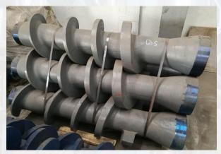
The extremely strong construction and shape of the screws facilitate fast induction of material at the inlet, and the gradual minor increase in screw thread gives increased pressure in the actual pressing zone. This ensures a high degree of pressing. The screws can be welded when worn to restore full thickness.
