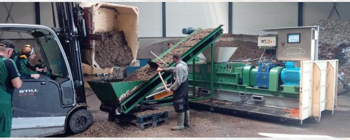
Mobile test plant makes it possible to test the efficiency of the Twin Press at the customer's premises.
