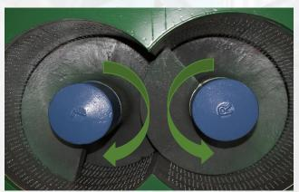
The way in which the Worm screws engage with each other and their internal opposing rotation prevents blockages and ensures constant kneading of the material under pressure. The result is uniformly pressed output with a high level of dry matter. Because no screw bearings are mounted at the outlet, blockage-free output is ensured.
