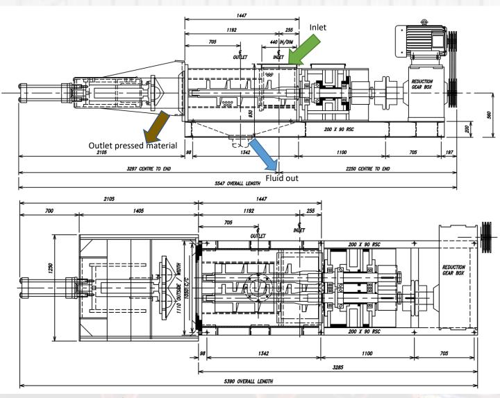
The Twin Screw Press is fitted with an automatically-controlled hydraulic backstop to ensure uniform dry matter.
