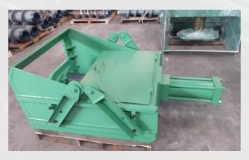
The hydraulic backstop can easily be removed for service
