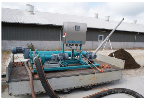
Mobile thickener systems, capacity 40-65 m 3 / h
