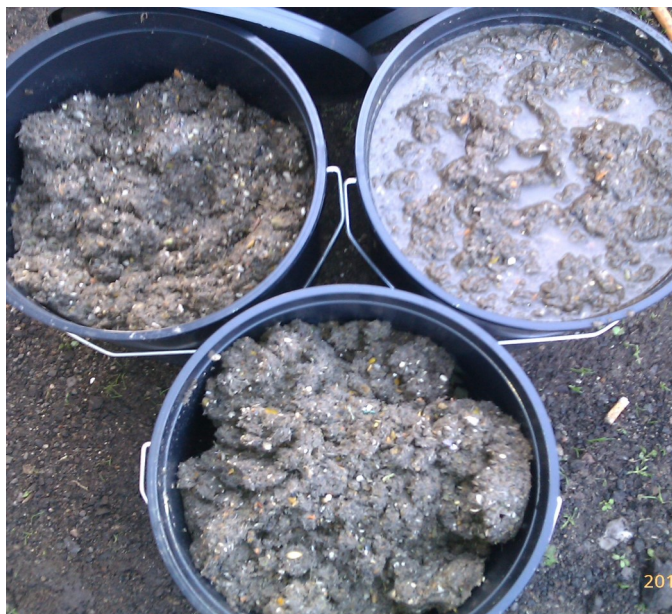
Organic pulp from waste after thickening Börger Bioselect. The pulp is concentrated from 6% ts. respectively to 12, 18 and 25% solids.
