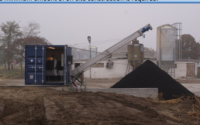
Container unit with fiber transport system as "plug and play" a minimum amount of on-site construction is required.
