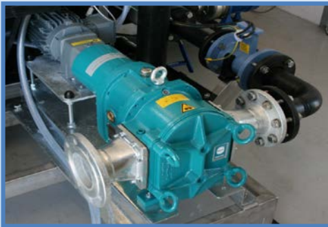
Biomass is introduced to the machine by variable drive pump, and flowmeter for control and documentation.
